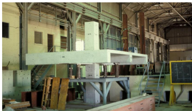
Development of design provisions for joints in RC structures subjected to seismic deformations
