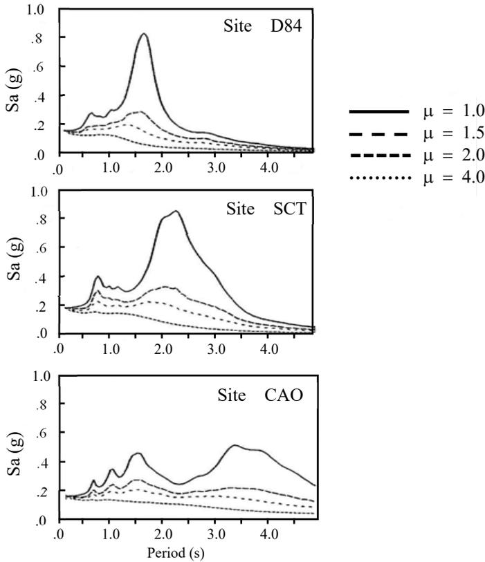
Figure 40. Response spectra that correspond to the mean values of simulated time histories, for different values of the ductility factor,  $\mu$ .
