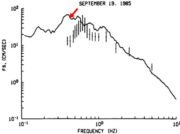
Figure 6. Comparison of observed and predicted values of the Fourier amplitude spectrum of the EW-SCT-850919 ground motion acceleration record (Mexico City, 1985; Castro *et al*, 1988)
