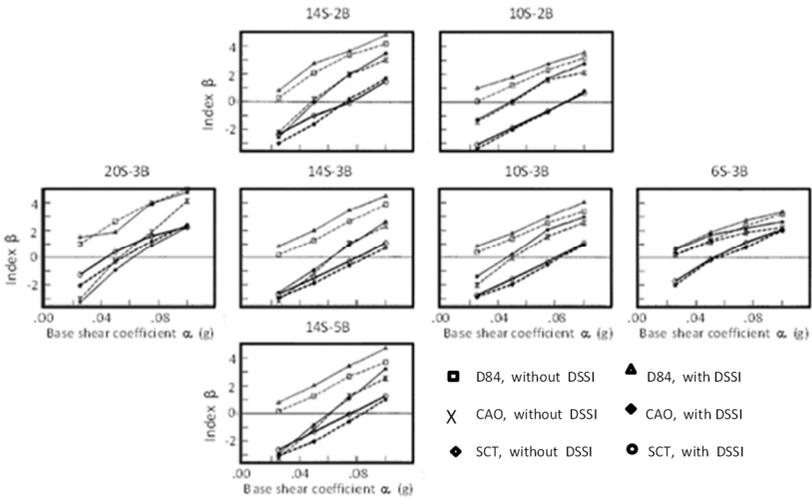
Figure 42. Reliability functions in terms of the base shear coefficient adopted for design at sites SCT, D84 and CAO.
