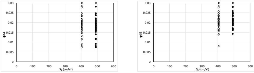
Figure 45. Values of the peak distortion  $\phi$  for a sequence of two earthquakes with intensities corresponding to a return interval of 250 years (Seven-story building)
