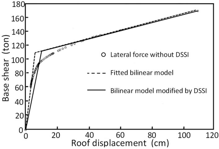
Figure 41. Force-displacement relation resulting from pushover analysis of the rigid- base structure, fitted bilinear model and fitted bilinear model modified by DSSI. Structure 14S-3B
