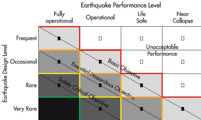
Figure 28. Expected performance vs seismic exposure (Calvi, 2010)
