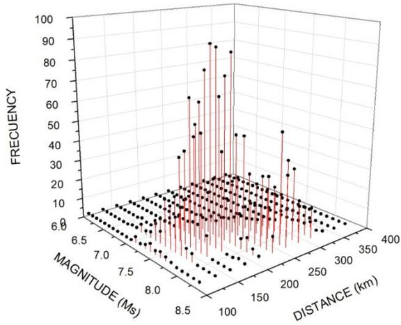
Figure 29. Joint probability density function of magnitude and distance for a given intensity at a site
