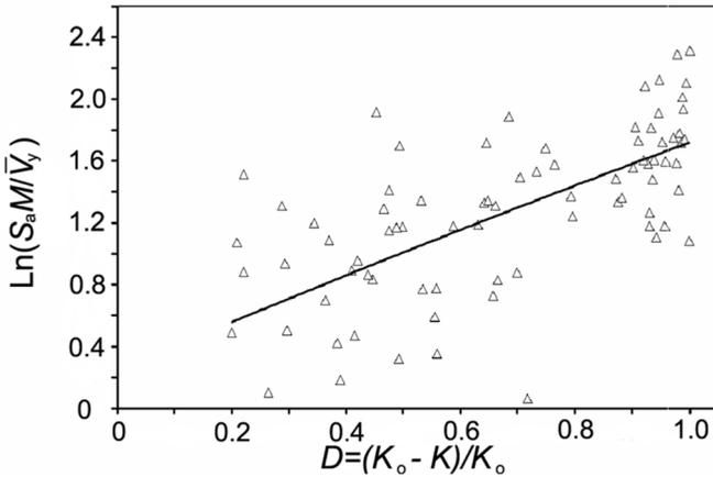
Figure 33. Reliability function in terms of normalized intensity for several twenty-story frame buildings
