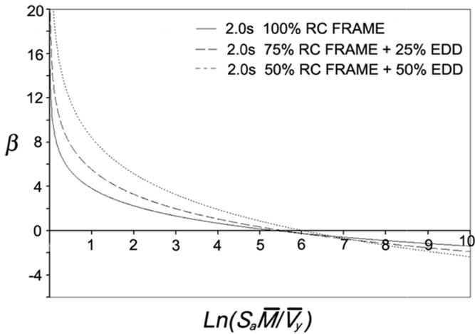
Figure 34. Normalized intensity vs  $\beta$  for 20-story system with energy-dissipating devices (EDD's) with EDD's
