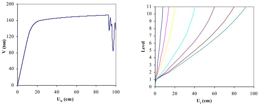
a) Base shear vs roof displacement for detailed model
