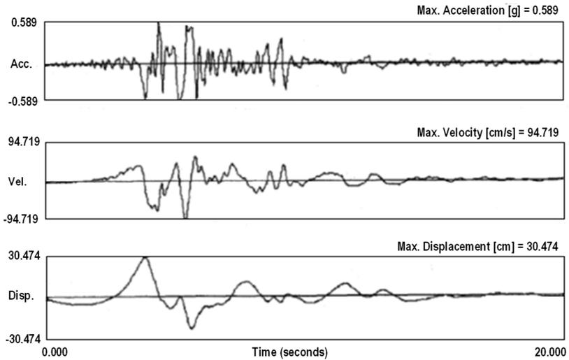
Figure 2. Ground motion time histories at Nehall County Fire Station (N-S) (Northridge, 1994) (Naeim, 1995)
