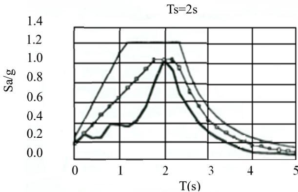
Figure 46. Uniform hazard spectrum for seismic intensities corresponding to a return interval of 125 years and proposed design spectrum
