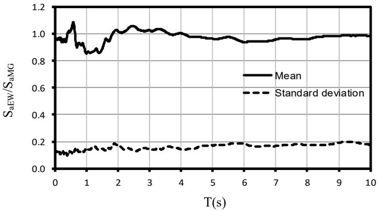
Figure 30. Relation of intensity of the EW component to the quadratic mean, for a sample of earthquake records
