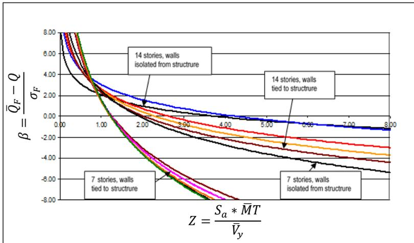
Figure 37. Seven- and fourteen-story frame buildings with walls tied-to and isolated-from the structure: different wall-stiffness values
