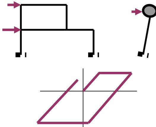
Figure 38. Systems with asymmetric shear-distortion functions
