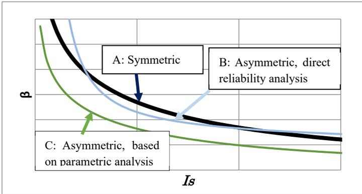
Figure 48. Seismic reliability functions for in-plan symmetric and asymmetric systems
