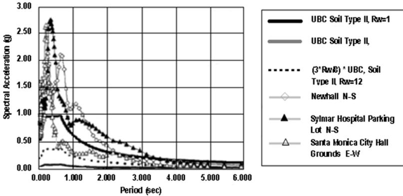
Figure 3. Elastic response spectra for selected Northridge 1994 records and UBC design spectra
