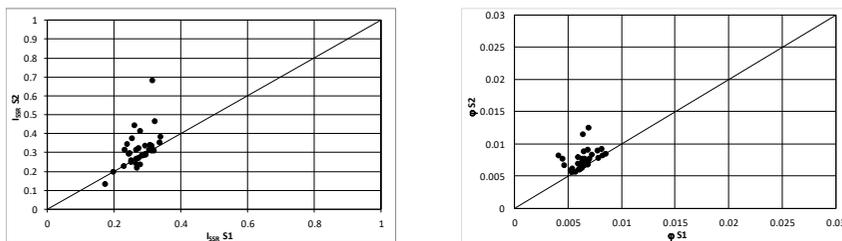
Figure 43. Response indicators obtained from results of dynamic response analysis of structures for intensities corresponding to a return interval of 125 years.
