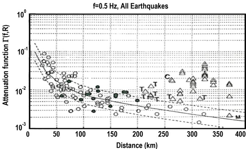
Figure 5. Evidence of amplification of earthquake spectra on the surface of volcanic rock formations (Mexico City, 1985; Ordaz and Singh, 1992)
