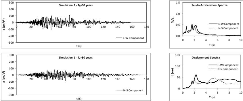
Figure 31. Simulated acceleration record for an intensity corresponding to a return interval of fifty years
