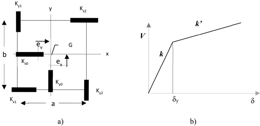
Figure 47. Simplified system used to represent a multistory in-plan asymmetric building: a) Plan, b) Shear-displacement functions of elements that provide the lateral strength
