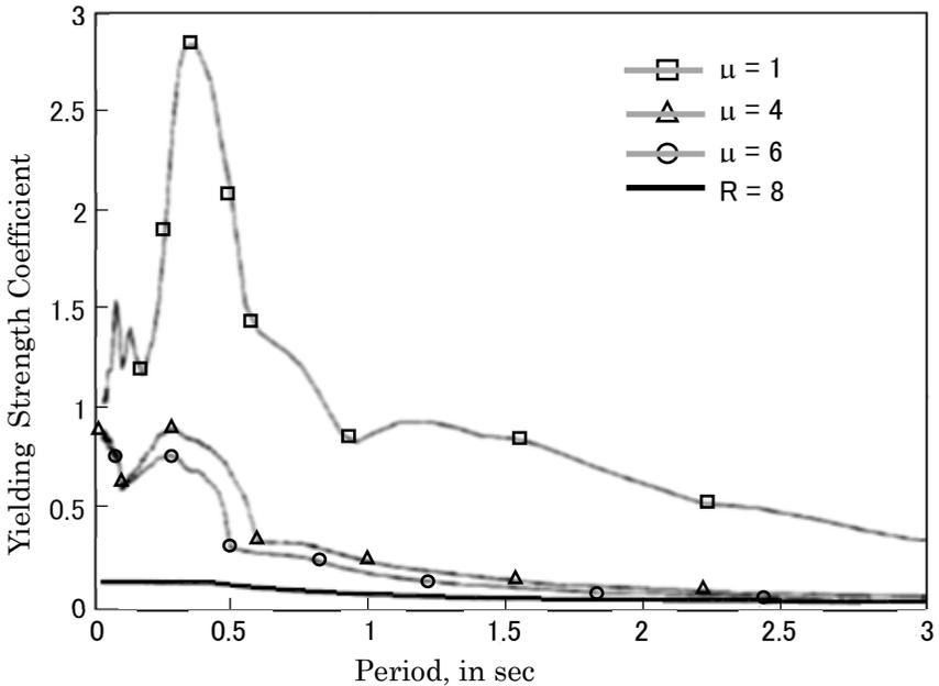
Figure 4. Inelastic response spectra (5 % damping) for the Sylmar Parking lot, compared with code design spectrum for an  $R_w = 8$  system (Northridge, 1994; Naeim, 1995)
