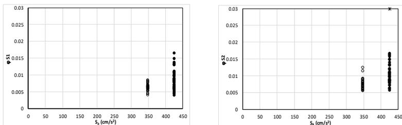
Figure 44. Values of the peak distortion  $\varphi$  for a sequence of two earthquakes with intensities corresponding to a return interval of 250 years (Ten-story buildings)
