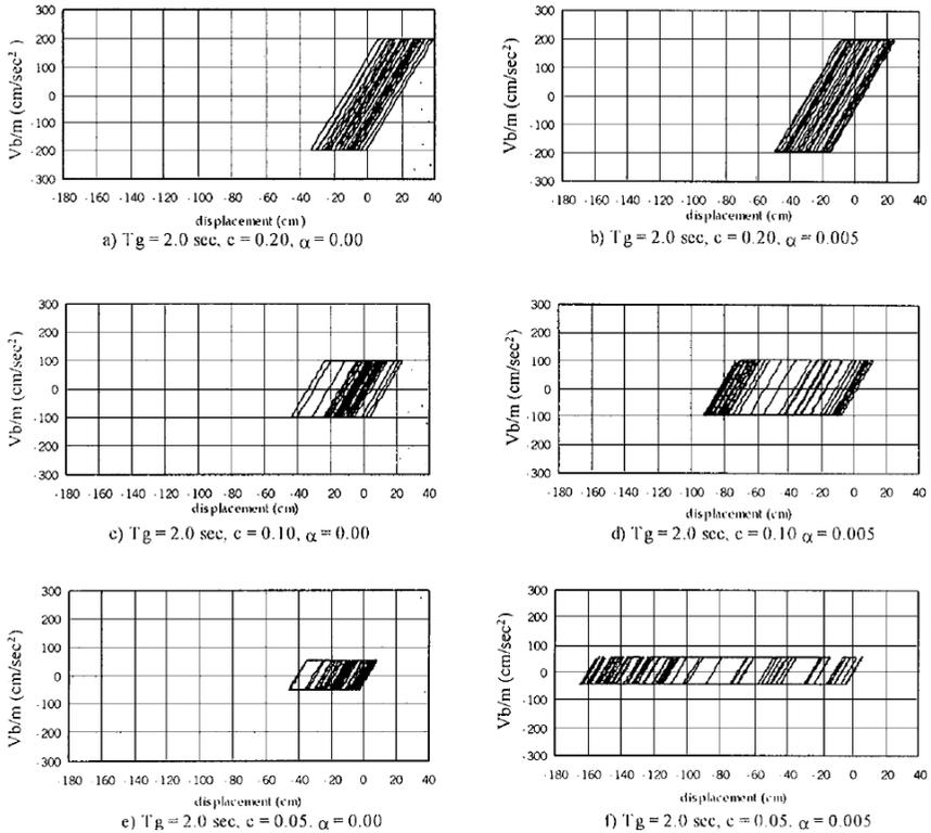
Figure 39. Cyclic response histories of systems with asymmetric shear-distortion functions (from Terán-Gilmore *et al*, 2000)
